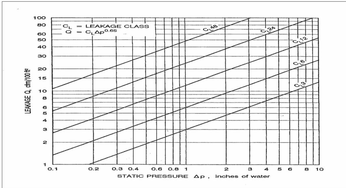
Prior to the 2013 version ASHRAE Standard 90.1 required Leakage Class 6 for rectangular metal and round flexible duct and Leakage Class 3 for round and flat oval metal duct.
